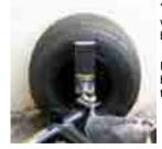
You can then place the kart on a flat level floor and check dynamic settings with the driver in the kart. Ensure the driver's legs do not obstruct the laser beams.
